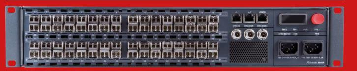
The MediorNet MetroN core router provides intense real-time signalrouting capacity (32x10G/32x4.25G ports) and offers non-blocking switching. The 2-RU device features switching delays of <40ms as well as high-speed re-routing that allows as many as 1,000 connections to be re-routed in less than a second.
